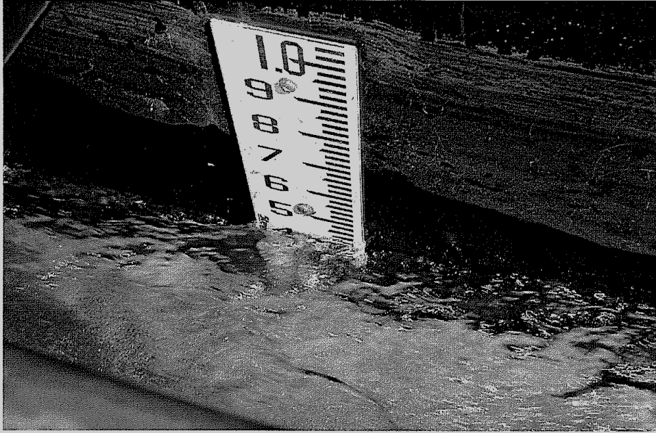
Image 4, upstream screen operating water depth
