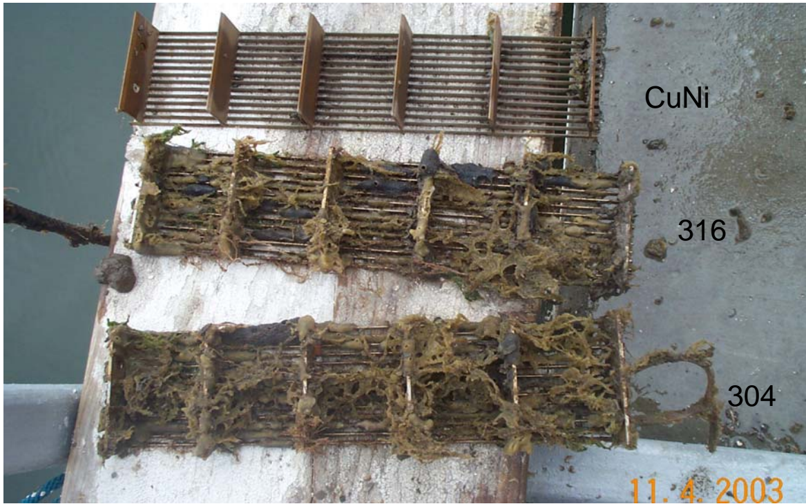
Figure 15. Photo shows Backside of Coupons at the Los Vaqueros site prior to cleaning. The CuNi coupon is free of biofouling after being in the water for five months. (Sample interval from 5/27/03 – 11/4/03)
